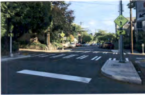
Rectangular rapid flashing beacons (RRFB) alert drivers at unsignalized intersections of people biking or walking.
